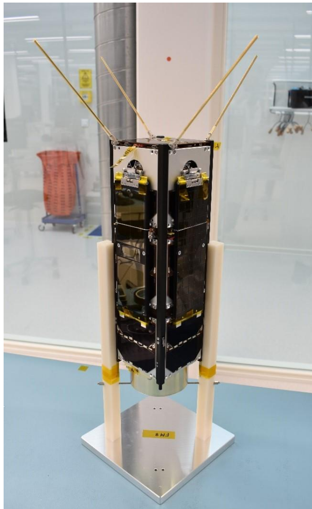
Fig. 4 Fully integrated flight model of SOAR.
