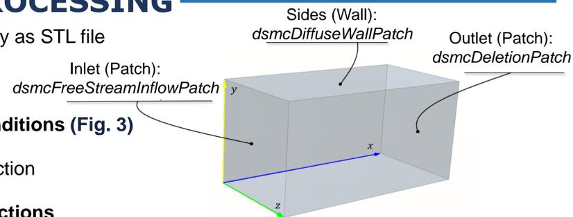
Fig. 3: Computational domain and boundary conditions set-up
