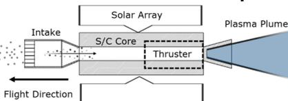
Fig. 1: Schematic of ABEP concept. Adapted from: [1]
