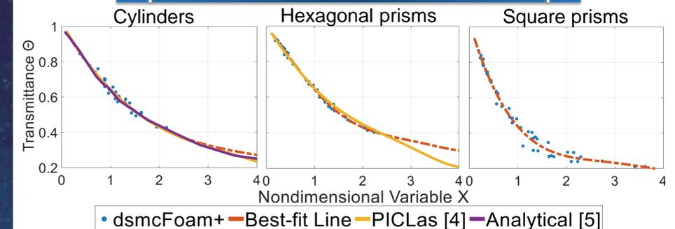
Fig. 6: Transmittance of cylinders (left), hexagonal prisms (centre) and square prisms (right)
