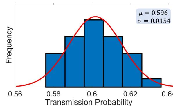
Fig. 4: Histogram and Gaussian distribution for transmittance of cylinder (L/R=1.4 and S=0)
