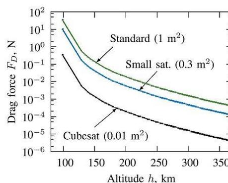
Fig. 1: Drag force over altitude for typical satellite sizes (cross sectional area) [17]
