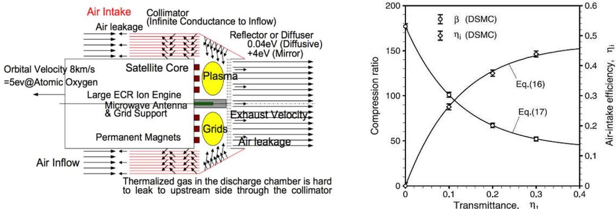
Fig. 11 Left: ABIE concept, Right: compression ratio and intake efficiency of ABIE [21]
