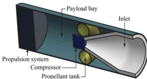
Fig. 7 RF Plasma Thruster Concept [5]
