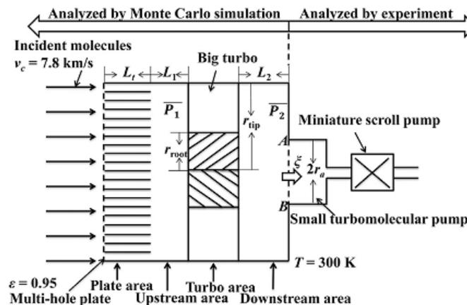
Fig. 18 Active vacuum intake [22]
