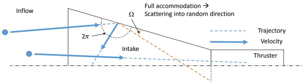
Fig. 10 Simple cone intake in free molecular flow
