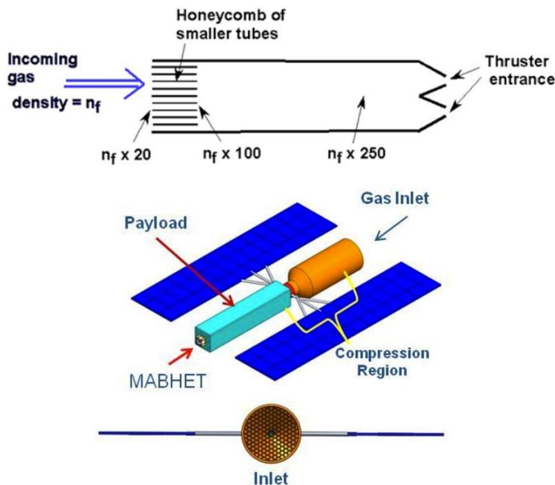
Fig. 14: MABHET, intake detail [12]
