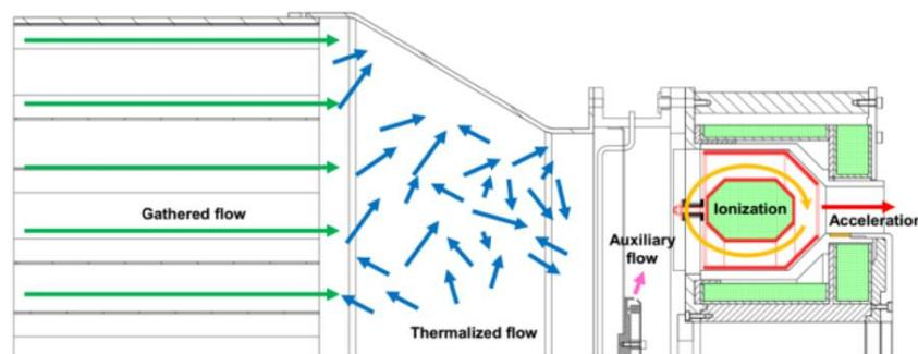
Fig. 21 SITAE L RAM-HET system scheme [19]
