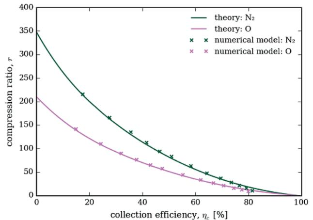
Fig. 17b: Intake compression ratio over collection efficiency for different gases and methods [20]
