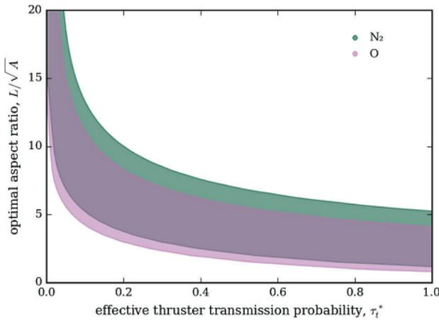
Fig. 17a: Optimal intake aspect ratio over effective, total transmission probability for different gases
