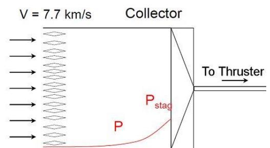
Fig. 12: ESA RAM-EP intake (based on [9])
