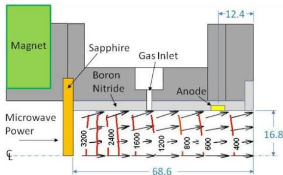
Fig. 5 Air-Breathing Cylindrical Hall-effect Thruster (ABCHT) [10]
